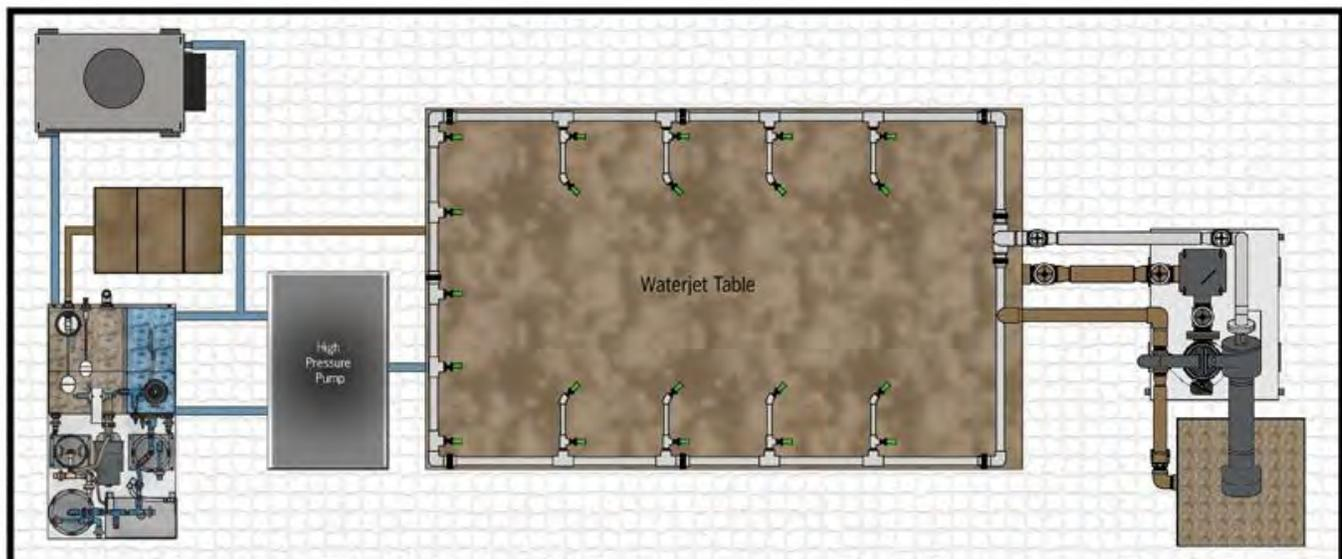
Closed Loop with Settling Weir & Chiller Typical Layout
