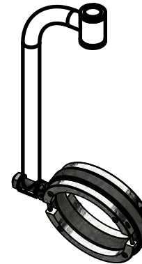
FITS TOOLS WITH TOOL BODY BETWEEN Ø4.625"-5.375"
